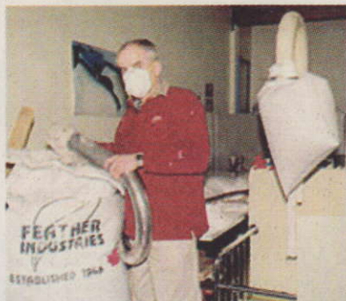
Adriaan filling a pillow. The machine to the right holds the pillow in place as it measures the weight. Below is Gwen sewing the pillow closed.
